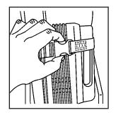
Remove the tire sealant and compressor kit strap by squeezing the two tabs of the quick release buckle.
